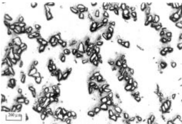
Fig. 9 Micrograph for A380Al/SiC (p) composites. Old material to new material of 3:1 weight ratio after third recycling with addition of Al-Si alloy
